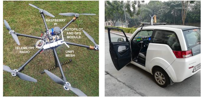
(a) Aerial node on a hexacopter. (b) Mobile ground node on a semi-autonomous car.
