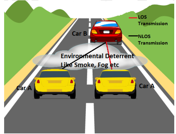
Fig. 1. VLC based V2V transmission model. Here, Car A with car headlamp as the transmitter, is trying to send information to Car B as the receiver, with the photodetector installed near its taillight.
