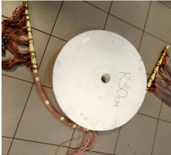
**Figure 4.** HTS cable during bending around the mandrel.
