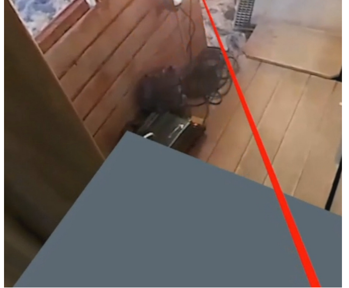
Fig. 3. A computer generated virtual floor (part of rectangle in lower part of image) rendered in 360-video of train waggon. The floor occludes parts of the scene and seems to float high above the floor in the video due motion parallax.
