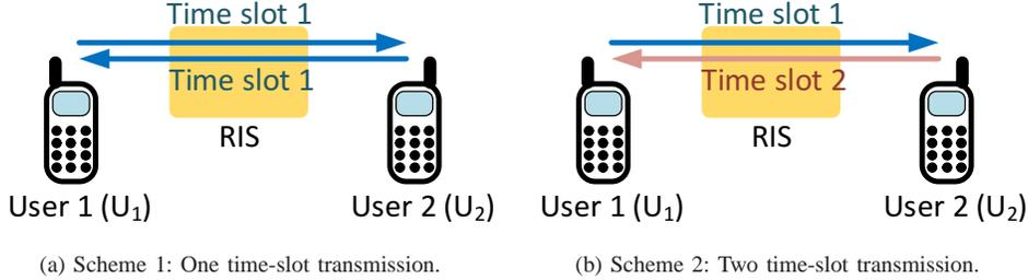
Fig. 1: Two possible transmission schemes for two-way communications.
