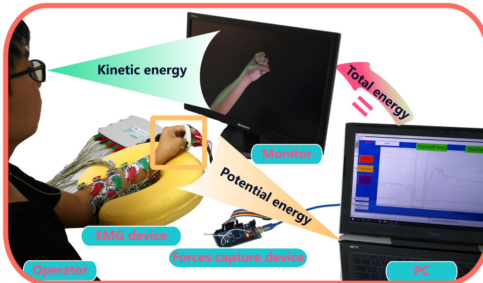
Fig. S2. Hardware structure for training states. The example of a hardware structure is composed of an EMG device, forces capture device, a PC, and a monitor. Note that, in the application, a smaller and general structure could achieve the frame of the myoelectric interface: electrodes, a microcomputer, and a motor unit.
