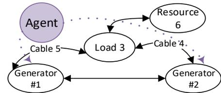
**FIGURE 4. THE SIMPLIFIED OCEAN GENERATION SYSTEM WITH TWO TURBINES SUPPLYING A LOAD.**
