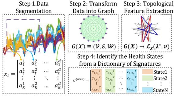
**FIGURE 2. DATA MANIPULATION & HEALTH ASSESSMENT USING GRAPH THEORETIC METHOD.**
