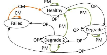
**FIGURE 3. THE MARKOV DECISION PROCESS OF OCEAN TURBINE WITH ASSOCIATED STATES.**
