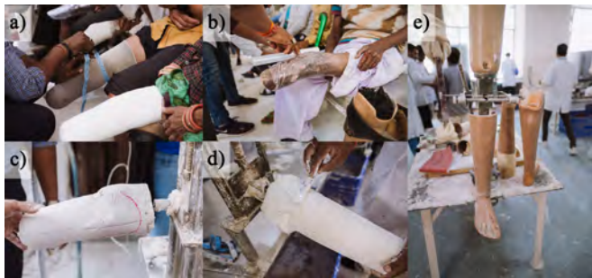
Fig. 3. Traditional process for manufacturing prosthetic limbs. a) Measuring key patient features. b) & c) Creating a plaster cast of an amputee's limb. d) Shaping the plaster limb cast. e) Manufacturing and adjusting final prosthetic socket
