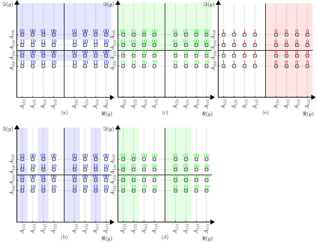
Fig. 4: NOMA constellation points for  $M = [4, 4, 2]$  showing the decision regions for: (a) first bit of  $U_1$ . (b) second bit of  $U_1$ . (c) first bit of  $U_2$ . (d) second bit of  $U_2$ . (e)  $U_3$ .
