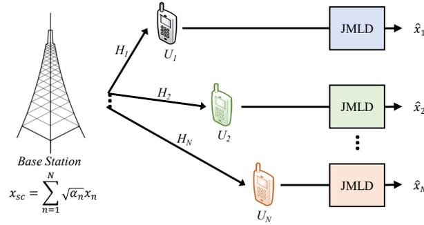
Fig. 1: Illustrative diagram of the system model assuming joint multiuser maximum likelihood detector (JMLD) at the receivers.
