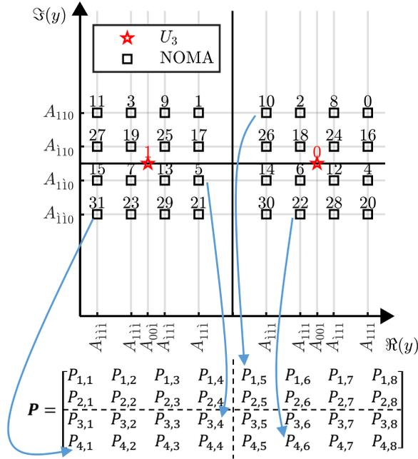
Fig. 3: Mapping NOMA constellation points to a scatter matrix  $\mathbf{P}$  for  $\mathbf{M} = [4, 4, 2]$
