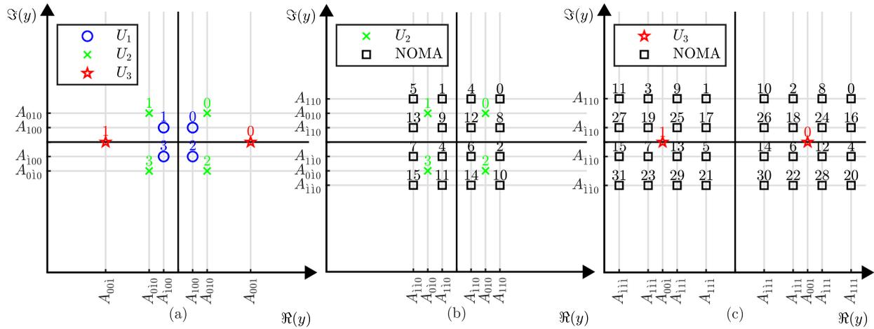
Fig. 2: Constellation points of: (a) All users without superposition coding. (b)  $U_2$  and the superposition coding between  $U_1$  and  $U_2$ . (c)  $U_3$  and the superposition coding among  $U_1$ ,  $U_2$  and  $U_3$ .
