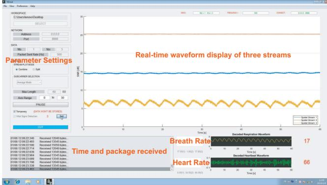
Fig. 7: Real time system's interface.
