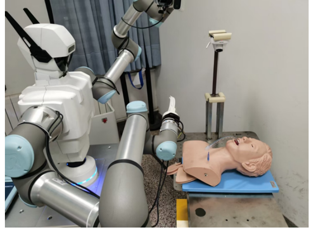
Fig. 10. The experiment platform includes a medical phantom, endotracheal tube, and AIRS, etc.
