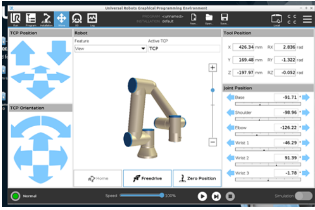
Fig. 3. State monitor interface shows the angle of each joint and allows doctors to remote-control or stop at emergency.
