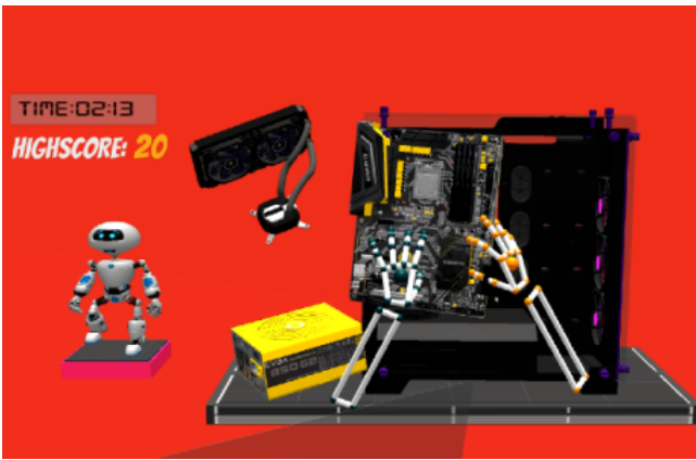
Fig. 12. Touchless hand interaction for learning PC assembly using leapmotion hand tracking
