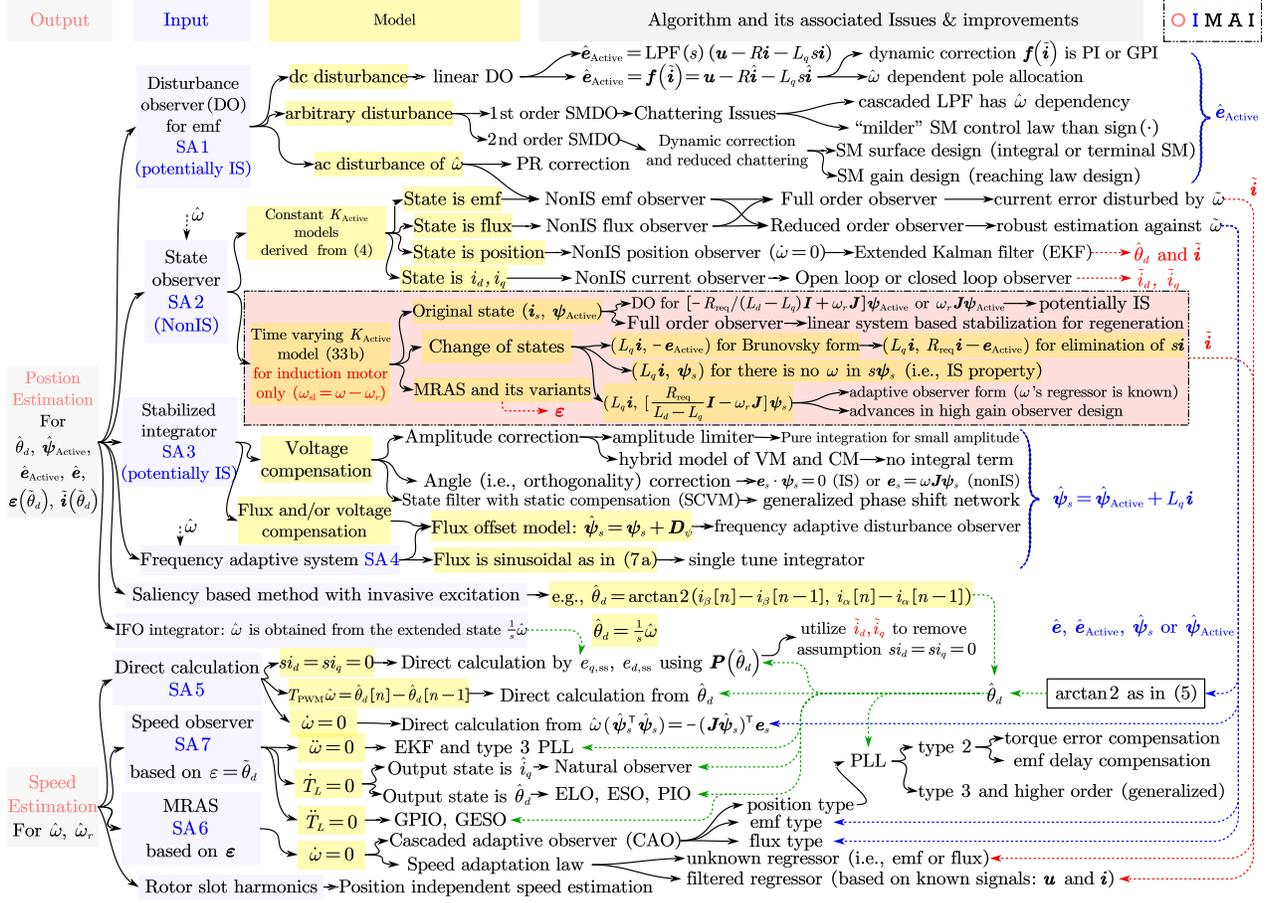
Fig. 4. The map of the overview by the 5 layer hierarchy “O-I-M-A-I”. Solid line means classification or logic flow, and dashed line describes the signal flow. The example saliency based method is [110]. Note the non-IS tuning and non-IS variants of SA1/3 discussed in Sec. III-B and III-C are not shown.
