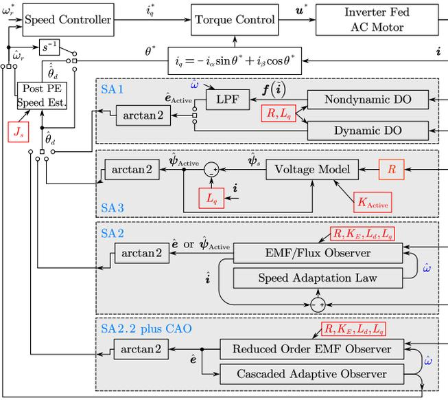
Fig. 3. Block diagram of the disturbance observer.
