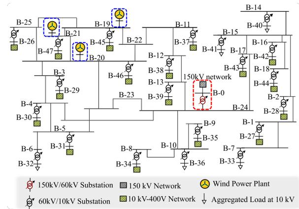
Fig. 1. Network topology for the 60 kV network in the DTU 7k-Bus Active Distribution Network indicating locations of the Wind Power Plants, and 10 kV-0.4 kV networks
