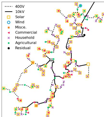
Fig. 2. The  $10\text{kV}$ - $400\text{V}$  network at Bus 27 illustrating  $10\text{kV}$  and  $0.4\text{kV}$  distribution lines, type of load profiles at each node, location of solar and wind power installations
