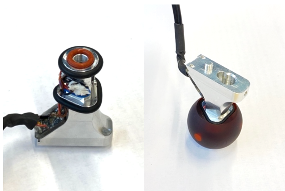
Figure 8. Improved triangle base design with head rotation lock allowing more precise sensor-magnet alignment for future use. (a) is without the head, viewed from the top/side, and (b) viewed from below, with the head fitted.
