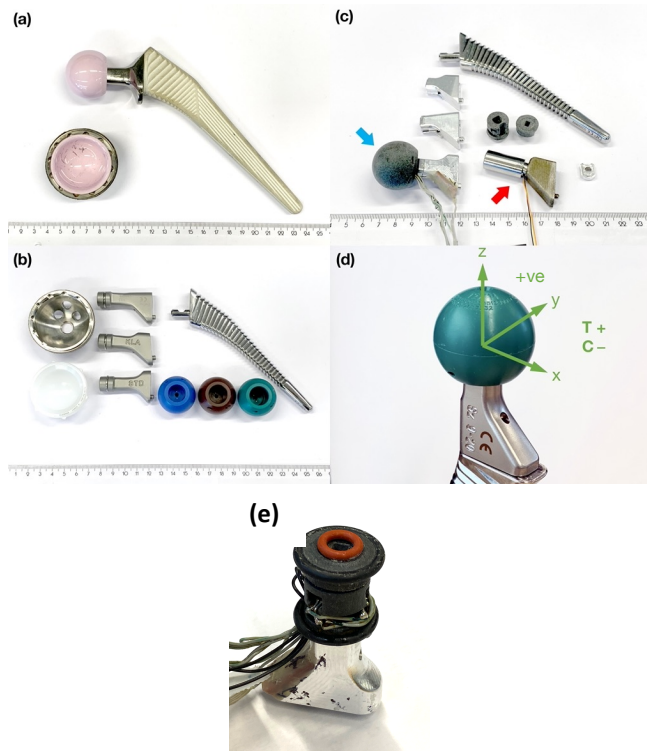
Figure 1. The stock implant (Corail Hip Systems, DePuy Synthes, Johnson&Johnson, Warsaw IN, USA) used as the starting basis for the design of the instrumented prototypes. (a) The permanent implant and (b) the temporary (trial reduction) implant with various modular neck and head geometries. (c) The instrumented prototype with instrumented necks and a modified head. Blue arrow indicating 3DOF prototype and red arrow indicating 1DOF prototype. (d) The coordinate system used in this report; tension (or compression from the negative side of the axis) is positive while compression is reported as negative. (e) The inside of the 3DOF implant with the head removed showing the radial and axial O-rings, sensor placement and wiring.
