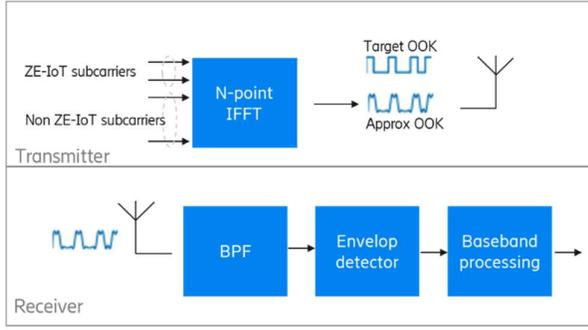
Figure 3: System illustration of ZE-IoT transceivers with OFDM-compatible OOK.
