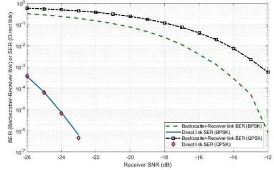
Figure 2: Bit error rate (BER) vs. the composite receiver SNR for the backscatter-receiver link amid a 30 dB stronger direct link signal assuming an additive white Gaussian noise channel for both links. Symbol error rate (SER) for the corresponding direct link is also shown.
