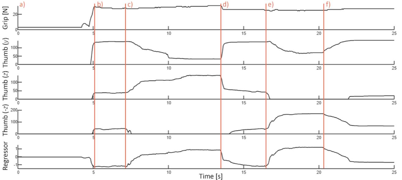
**Fig. 3** Visual example of the relation between each sensor value and regressor output across grasp and pull movements. a) grasping object, b) neutral grasp, c) pulling object to the right until slip, d) returning to neutral grasp, e) pulling object to the left until slip, f) returning to neutral grasp.
