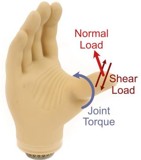
**Fig. 1** The Ottobock SensorHand Speed system includes sensors measuring normal (light red) and shear loads (dark red) at the tip of the thumb, and joint torque (blue) at the thumb joint.
