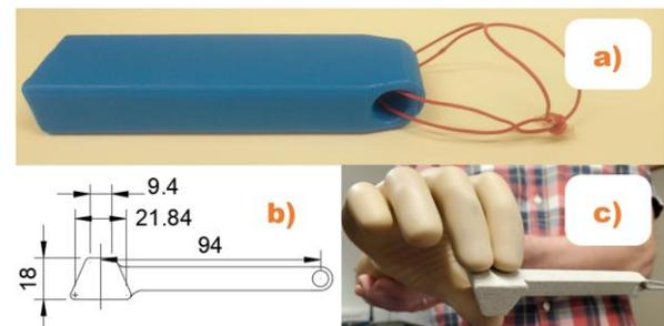
**Fig. 2** a) Training block, b) trial totem detail [mm], c) view of trial totem grasped by prosthetic before a pull attempt.
