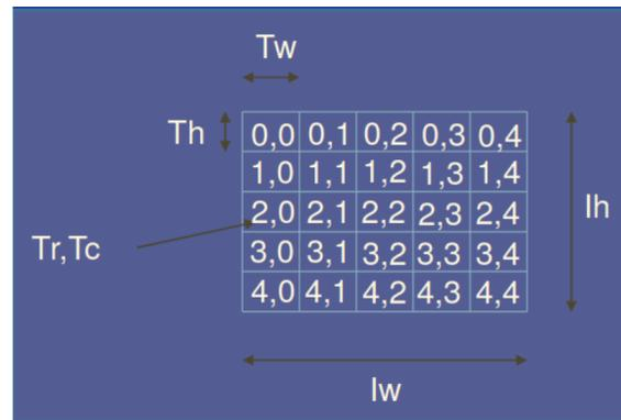
Fig. 10. Mapping of an image to individual tiles.  $T_w$  indicates Tile width,  $T_h$  indicates tile height,  $T_r$  indicates tile row,  $T_c$  indicates tile column,  $l_h$  indicates image height and  $l_w$  indicates image width.
