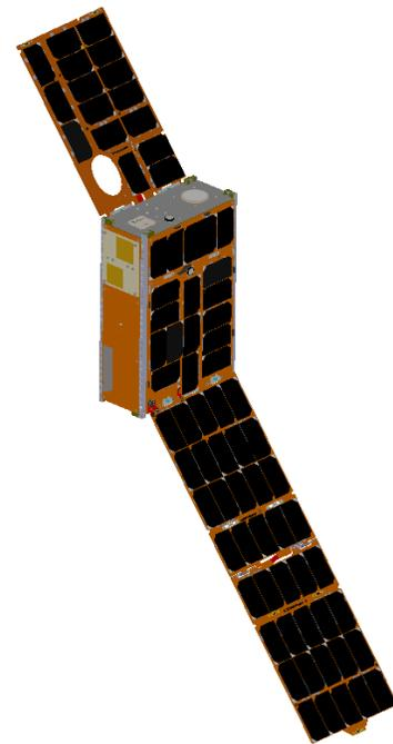
Fig. 1. CAD drawing of CogniSAT-6.
