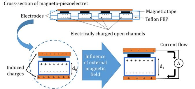
Fig. 1. Schematic representation of the magnetic-piezoelectret and how their macroscopic dipoles, changes under the influence of an external magnetic field.
