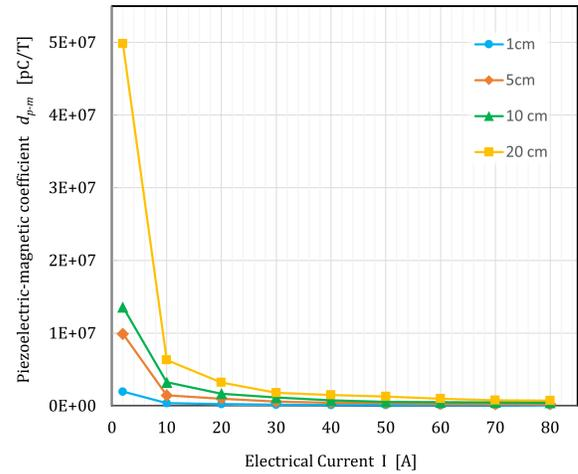
Fig. 6. Piezoelectric-magnetic coefficients ( $d_{p-m}$ ) measure for different electrical current values and for the four distances between the transducer and the electrical wire considered in this study (1, 5, 10 and 20 cm).
