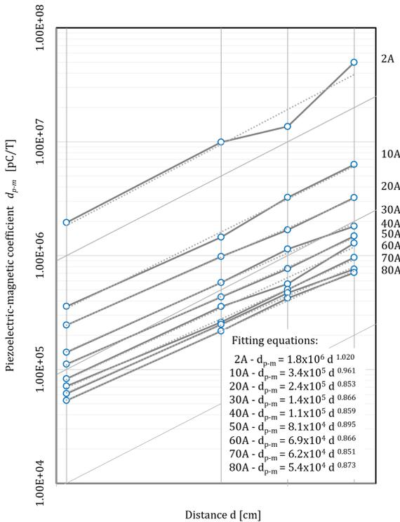
Fig. 8. Piezoelectric-magnetic coefficients ( $d_{p-m}$ ) versus transducer-wire distance.
