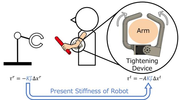
Fig. 2. Schematic diagram of how to present the stiffness of robot to human.  $K_p^r$  is the stiffness gain of the robot.  $\Delta x$  is the difference between the current and target angle.  $A$  is the variable that is applied to feel the force of the tightening device.
