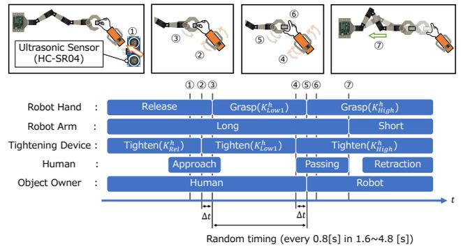
Fig. 3. Experimental scenario for H2R handover. Each scene of H2R handover (top) and state transition diagram (bottom). Random time assumes the robot is not guaranteed to move simultaneously every time.
