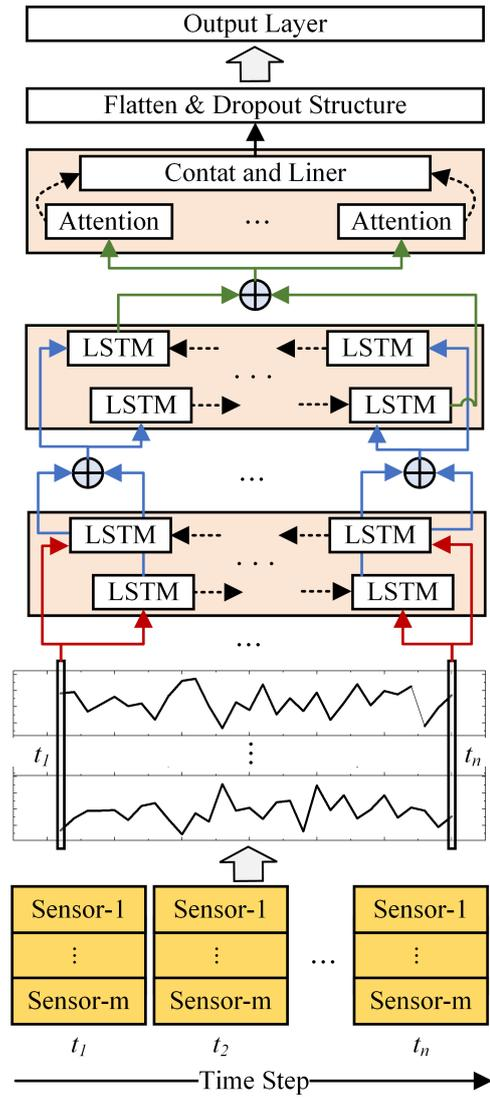
Figure 6. Structure of general prognostics DL model.
