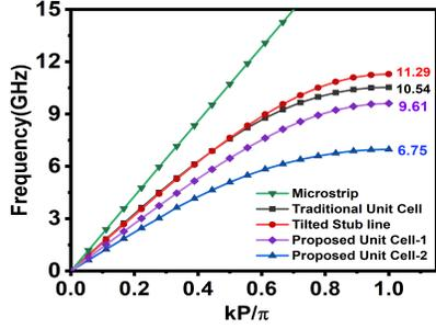
Fig. 2. Dispersion characteristics of different SSPP unit cells.
