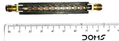
Fig. 12. Photograph of fabricated SSPP LPF.
