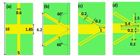
Fig. 1. Unit cell structures of (a) traditional SSPP unit cell, (b) tilted stub SSPP unit cell, (c) proposed unit cell-1, and (d) proposed unit cell-2. (dimensions unit: millimeter)
