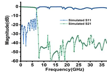
Fig. 10. Simulated S-Parameters of the proposed filter.
