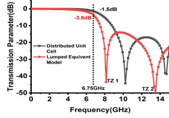
Fig. 5. Transmmission parameter of distributed and equivalent lumped circuit SSPP unit cell.
