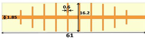
Fig. 7. Schematic configuration of traditional SSPP LPF.(unit: millimeter)
