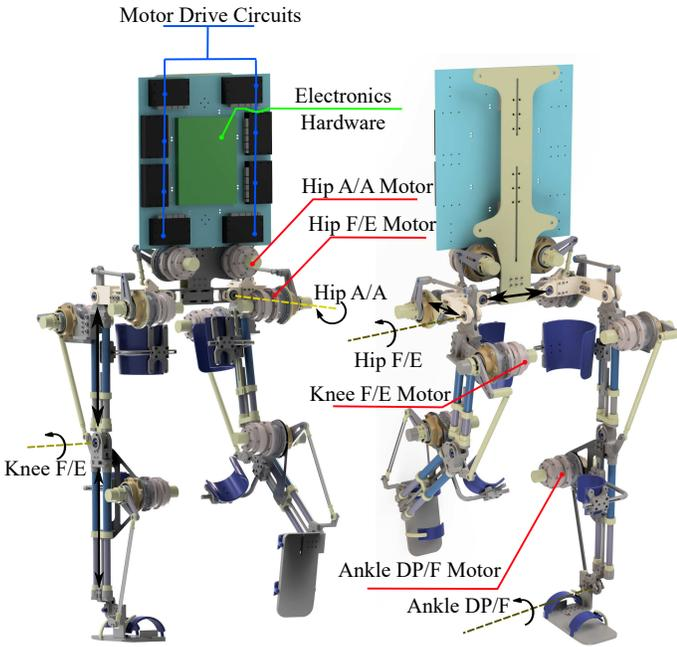
Fig. 2: Joint configurations of the exoskeleton Co-Ex.
