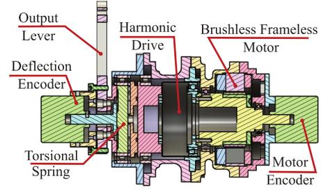
Fig. 7: Series elastic actuator unit, CAD model.
