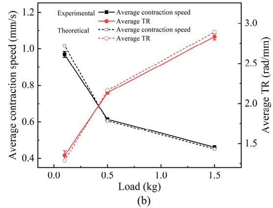
Fig. 5. The performance test results of the proposed TSA-based CVT. (a) The experimental and theoretical load contractions for the proposed TSA-based CVT varied with the number of turns of the motor, maintaining a constant output speed of 12.5 rpm/min, while carrying workloads of 0.1 kg, 0.5 kg, and 1.5 kg, respectively. (b) The experimental and theoretical average contraction speed of load and average TR varied with the load, maintaining a constant motor output speed of 12.5 rpm/min.
