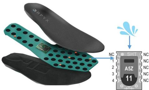
**Fig.4** temperature-humidity based insole systems and inside elements
