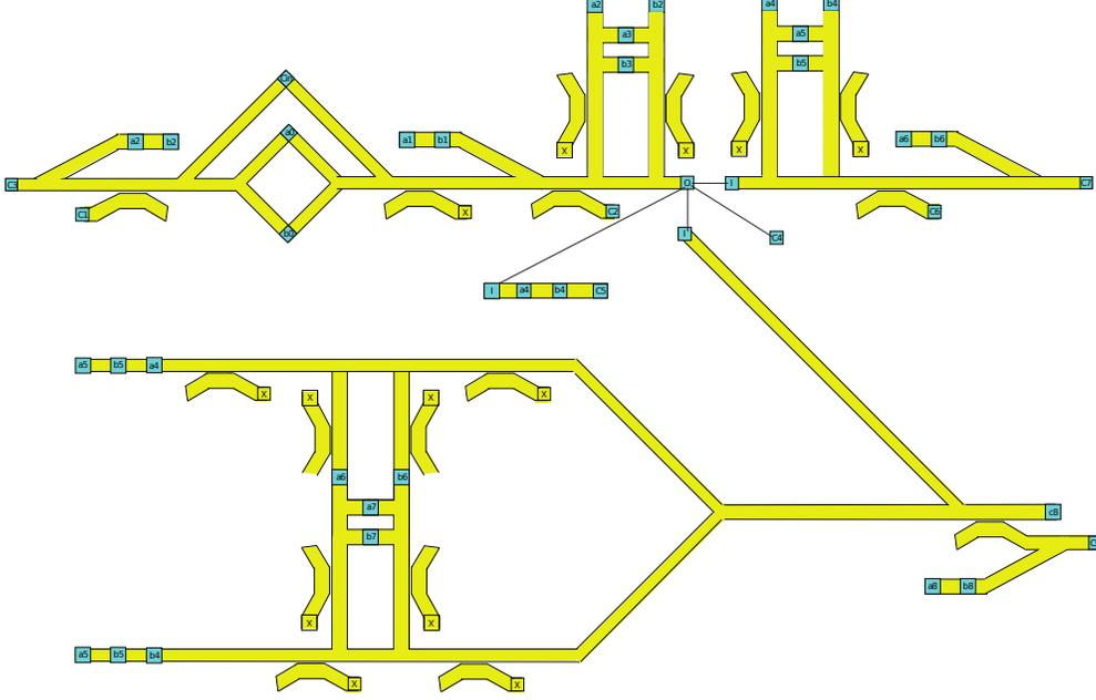
FIG. 5. Carry-out1 to Carry-out9 Calculation using Normalizers and Converters. energy consumption  $E_{SW} < E_{CMOS}$ , and based on this, we can determine the performance constraint that the transducer needs to fulfil.
