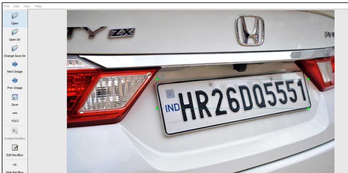
Fig 9. The LabelImg software being used over image in [Fig 7].
