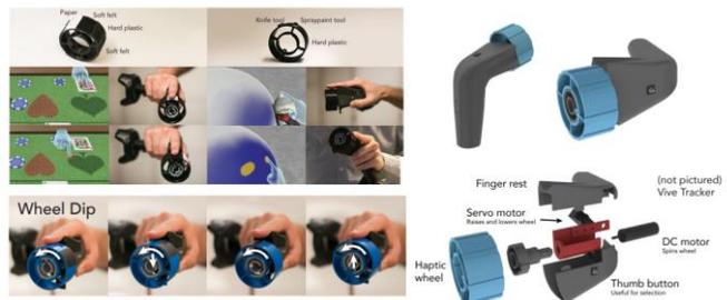
**Fig. 4. Haptic Revolver.** Examples of use and configuration.
