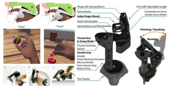
**Fig. 5. CLAW.** Prototype and examples of the haptic renderings inside VR.
