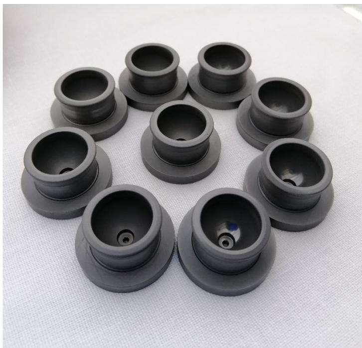
Figure 5. Set of parts with Cu – CuMo<sub>6</sub>S<sub>8</sub> coating.
