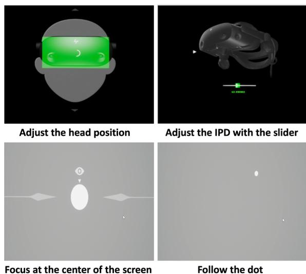
Fig. 5: Before starting the VR application, participants performed a calibration for the eye-tracking to ensure optimal data accuracy. The procedure involved (a) adjusting the head position, followed by (b) setting the interpupillary distance (IPD) using the slider. Subsequently, (c) participants focused on the center of the screen, and finally, (d) they were instructed to follow the dot.
