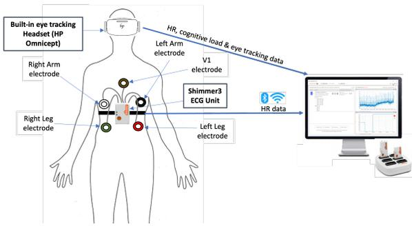
Fig. 3: Hardware setup and electrode placement: A wireless Shimmer3 ECG system employing Bluetooth and WiFi for heart rate data streaming. The Shimmer kit collected data using ConsensusPRO software. The HP Reverb G2 Omnicept has a built-in eye-tracking headset and other sensors that were used to gather participants’ heart rate, cognitive load and eye-tracking data.
