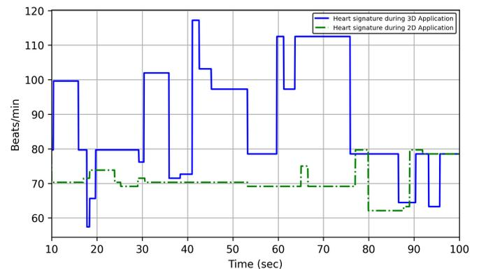
Fig. 1: Comparison of a participant's heart rate from Radar sensor during 2D application and 3D immersive virtual reality environment.
