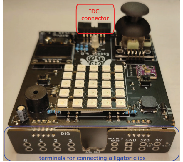
Fig. 4. Close-up view of the connection terminals of the BitDogLab that can be connected with alligator clips.
