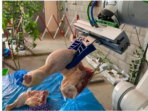
Fig. 9: Example picture of the Festo gripper that adapted to the shape of the chicken piece to firmly grasp it during the picking and placing operation in one of the experiments.
