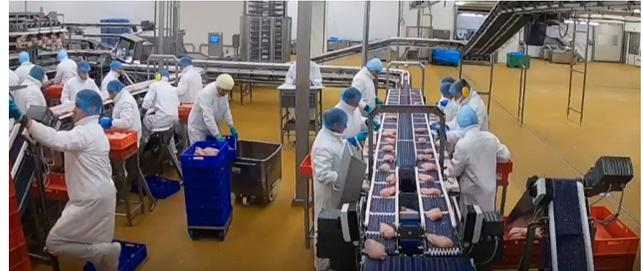
Fig. 1: Poultry pieces are currently manually segregated from cluttered piles in bins to place them in order on the conveyor belt by human laborers for further processing in the processing line in an industry that is still labor intensive (source: [3]).
