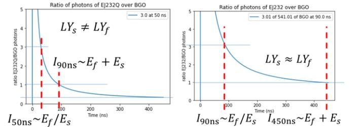
Fig. 2. (left) ratio of total produced photons between EJ232Q and BGO as it develops over time. When this ratio crosses 1, energy sharing is not visible in the integral histogram, while when this ratio is more than 1, strongly shared events are favored according to the ratio value; and (right) when the light yields are substantially the same, the ratio converges to 1 with time.
