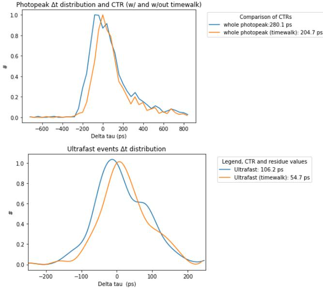
Fig. 5.  $\Delta t$  distributions from the 3:1  $3 \times 3 \times 15$  mm<sup>3</sup> BGO:EJ232 metapixel: (top) the whole photopeak is fitted with a hybrid Gaussian-Laplacian fit before and after timewalk correction; and (bottom) A 9.5% of chosen shared events, corresponding to the blue population of figure 4, fitted with a hybrid Gaussian-Laplacian function before and after timewalk correction.
